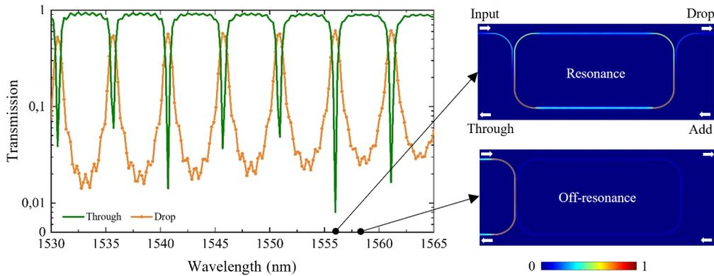
**Fig. 2** Transmission spectra of add and drop ports of the MEMS filter obtained from 3D FDTD simulation in the Filter-ON state (passive state). At the right, optical power profiles are shown for the resonant and off-resonant wavelengths.
