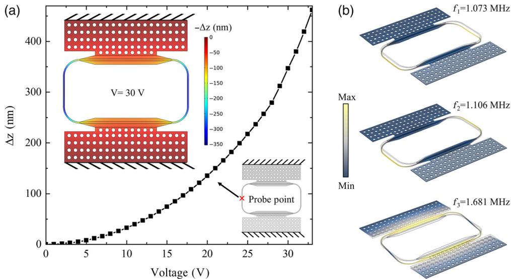
**Fig. 3** (a) Electromechanical simulation results showing the actuation curve of the micro-ring resonator. The vertical displacement of the ring for  $V = 30$  V is demonstrated in the inset. (b) Three first eigenfrequencies of the MEMS micro-ring resonator.
