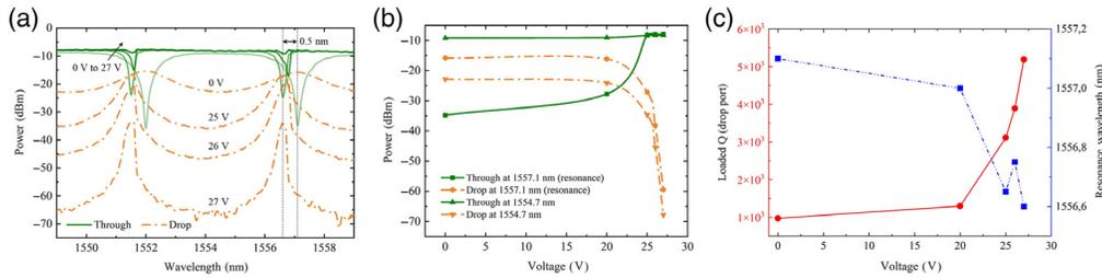
**Fig. 8** (a) Power spectra of the drop and through ports of the MEMS add-drop filter. (b) Actuation curve of the device at  $\lambda = 1557.1$  nm (on-resonance) and  $\lambda = 1554.7$  nm (off-resonance). (c) Resonance wavelength shift and the loaded  $Q$  factor (drop port) versus the actuation voltage.
