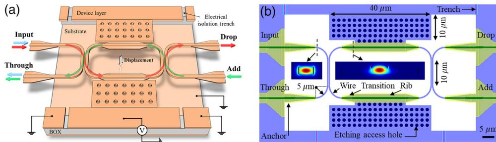
**Fig. 1** (a) Schematic representation of the MEMS add-drop filter (not to scale). The device is tuned by actuating the vertically movable suspended ring resonator and (b) layout of the device with the scaled dimensions. Optical mode profile in the fully etched and shallow etched waveguide sections are shown in the inset. No color code relation is applied between the two figures.
