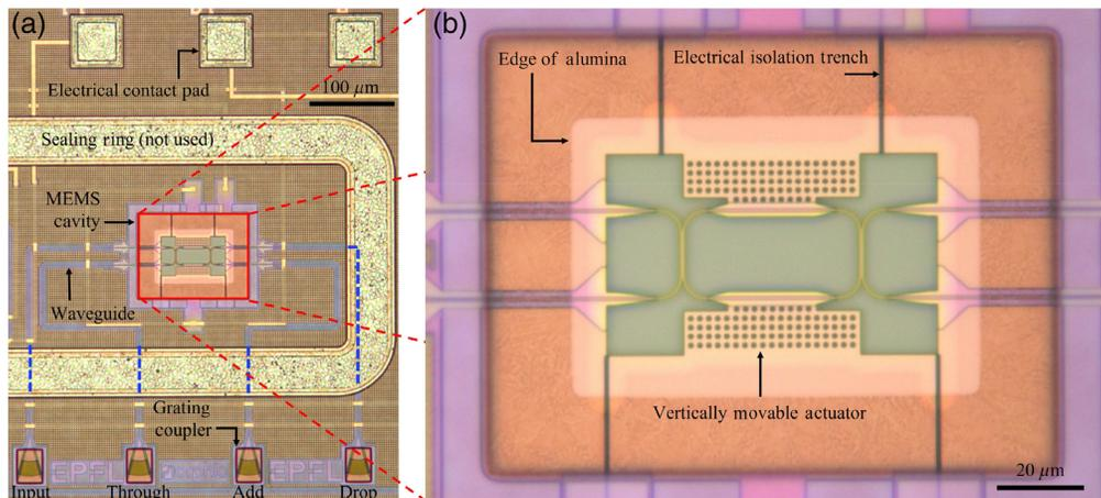
**Fig. 5** Optical microscope image of the chip area after vapor phase hydrofluoric acid MEMS release. (a) Successful integration of the MEMS device in the full stack of iSiPP50G platform next to the grating couplers and the electrical bond pads. (b) Closer view of the released MEMS micro-ring resonator filter.
