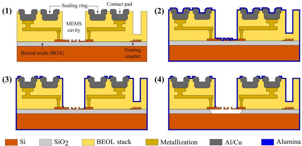
**Fig. 4** Post-processing steps for releasing the silicon photonic MEMS components: (1) starting stack after preparatory removal of the remaining oxide on and between the waveguides, (2) alumina passivation by ALD, (3) alumina patterning by dry/wet etching, and (4) VHF release etch to remove the BOX.
