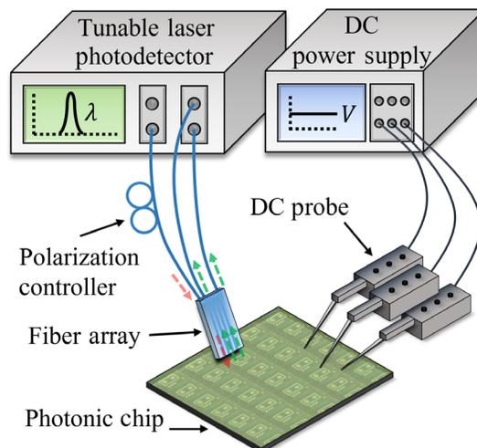
**Fig. 7** Schematic of the characterization setup.
