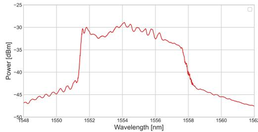
(e) Optical spectrum of the mode-locked laser.
