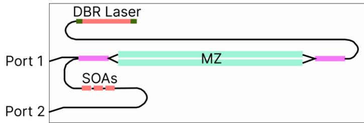
Figure 2. Simplified overview of the chip used for measurements. Light from a DBR laser is guided towards an MZ modulator that can guide the light either towards Port 1 or towards an SOA section containing three SOAs. From the SOAs the light is guided towards Port 2.
