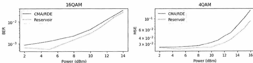
Fig 4. Testing results showing BER for 16 QAM and MSE for 4 QAM for a range of fiber input powers
