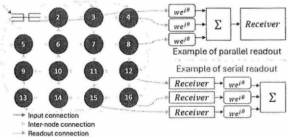
**Fig. 1:** 16-node reservoir with 2 possible readout schemes. Nodes are numbered vertices, with the exception of node 1, shown as an abstracted 3x3 multimode interferometer.
