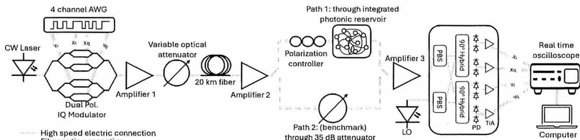
**Fig. 2:** Experimental setup. CW: continuous wave laser, AWG: arbitrary waveform generator, LO: local oscillator, PBS: polarization beam splitter, PD: photodiode, TIA: transimpedance amplifier.
