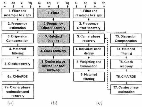
Fig. 3: DSP for (a) benchmark (b) photonic RC with parallel readout, (c) photonic RC with serial readout.
