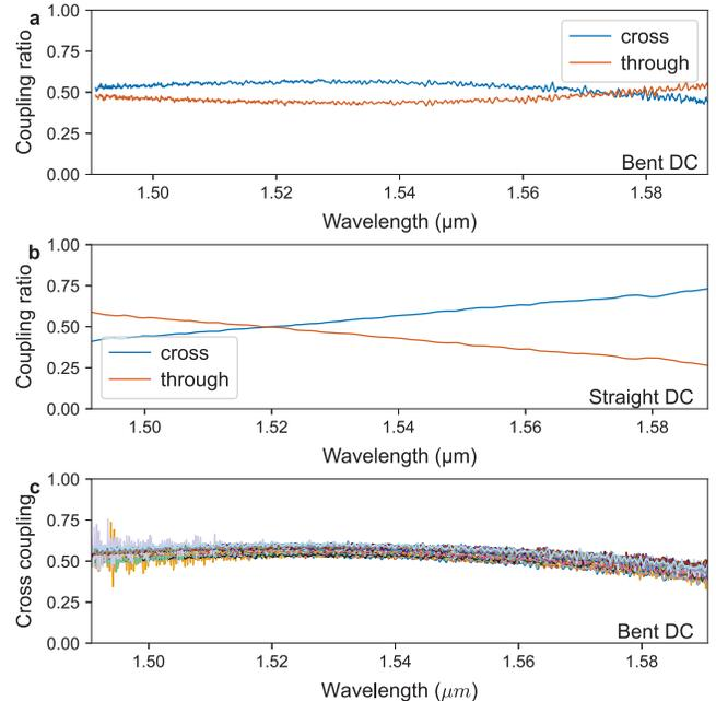
Fig. 2. The measured coupling ratios of the bent DC (a) and straight DC (b) along with the cross coupling spectra for bent DC over 63 measured dies in a 300 mm wafer (c), where each color represents one die.  $3.7\times$  less coupling variation is observed in the bent DC as compared to the straight DC. Robust performance of the bent DC is observed over the wafer.
