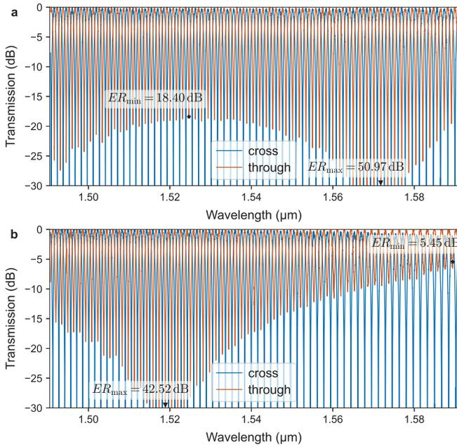
Fig. 3. The proposed MZI spectrum based on bent DCs (a), and the traditional MZI spectrum based on straight DCs (b). Minimum and maximum ER values are marked. At least  $2.7\times$  improvement in the ER wavelength operational range for the proposed MZI is shown. The free spectral range for both MZIs is designed to be 100 GHz.
