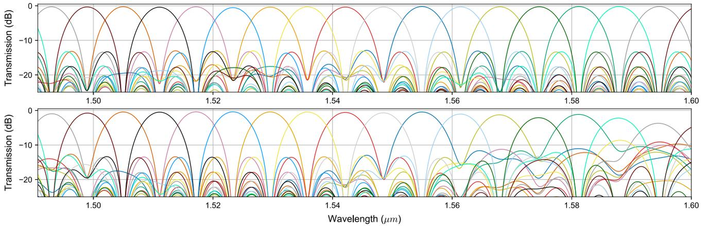
Fig. 6. 16-channel cascaded MZI WDM spectrum, with 800 GHz channel spacing, based on the measured bent DC (a) and straight DC (b) calculated using the transfer matrix method. Significant improvement is observed in channels isolation and insertion loss for the WDM system based on bent DCs.
